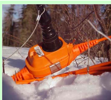
A Sercel Field Digitizer Unit (FDU) is a single channel acquisition unit to which the geophone string is directly connected. One or more FDU's are integrated into the cable, making up a Link.
