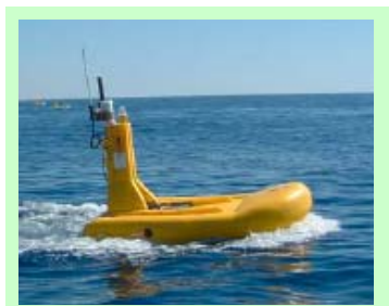
Seamap's BuoyLink uses GPS to track multiple seismic gun floats and tail buoys.
